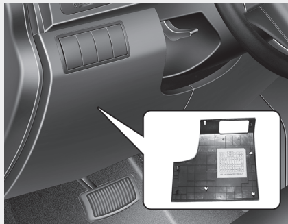
Inner fuse panel
