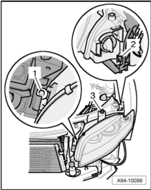
Fig. 373: Locating Screws Courtesy of VOLKSWAGEN UNITED STATES, INC.
