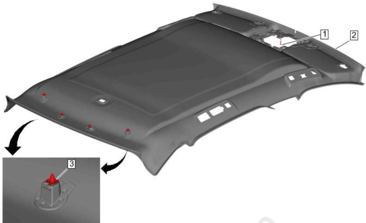
Fig. 15: Roof Console Bolt
