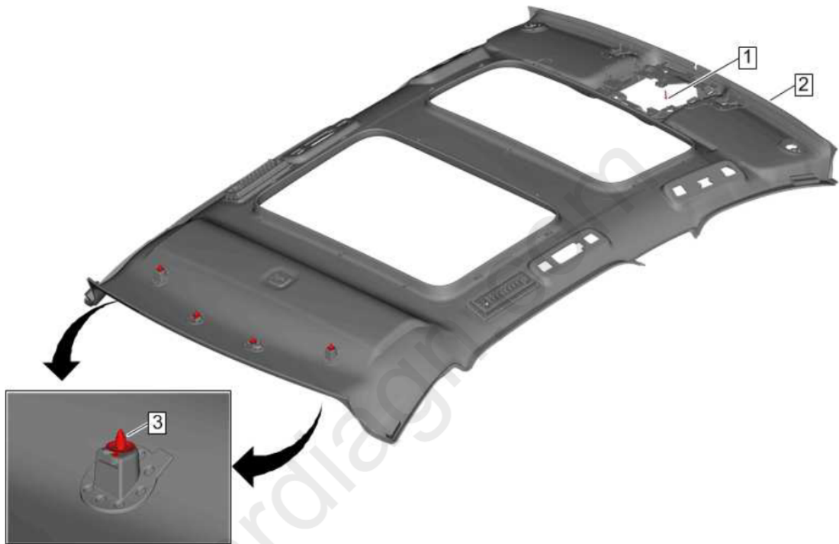
Fig. 38: Roof Console Bolt
