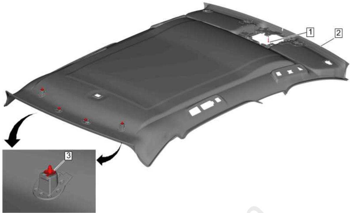
Fig. 14: Roof Console Bolt
