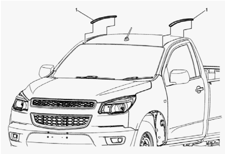
Roof Panel Joint Finish Molding Replacement
